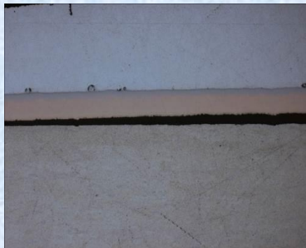
4- 2.5 mils Cu+ Ni delamination
