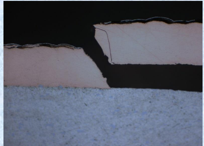
5- 2.0 mils Cu, Failure, no delamination
