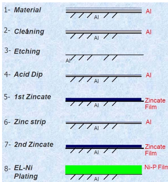
Figure 1 - Zincate process steps.
