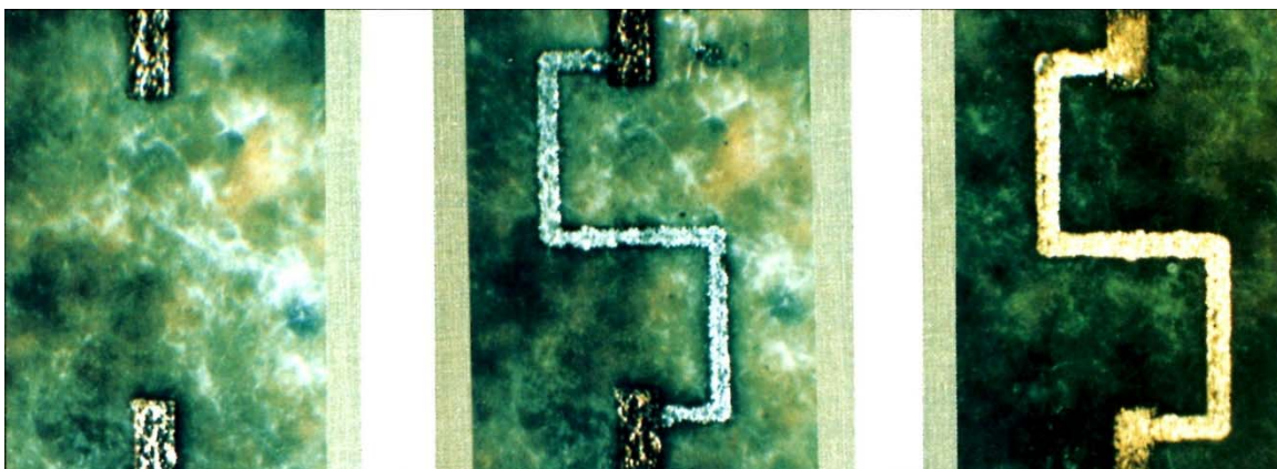
Figure 13 - Example of customized interconnections made with laser seeding and self-induced repair: (1) two leads with a spacing of 0.2 mm; (2) after seeding with palladium, resistance is about 100 ohms; (3) after self-induced repair, resistance is about 50 mohms.
