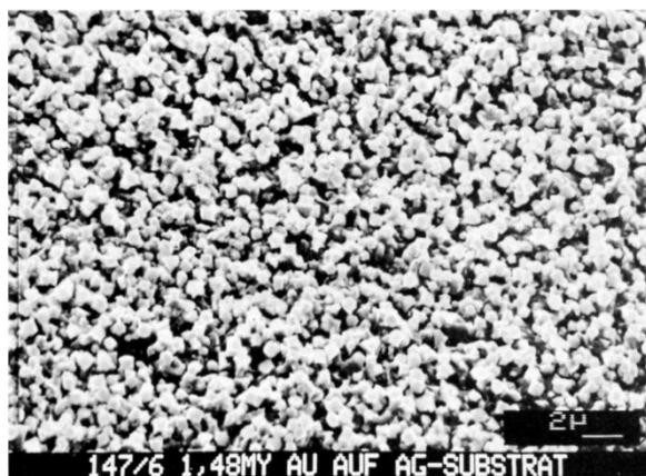
Figure 12 - SEM of gold deposited from Bath EL1 (10 g/L KCN, 80°C) on silver.
