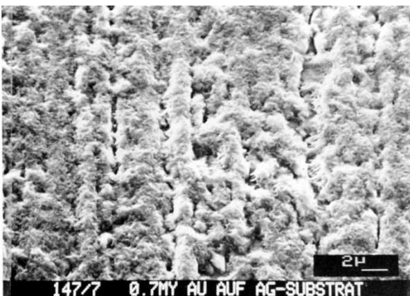
Figure 11 - SEM of gold deposited from Bath EL1 (15 g/L KCN, 80°C) on silver.
