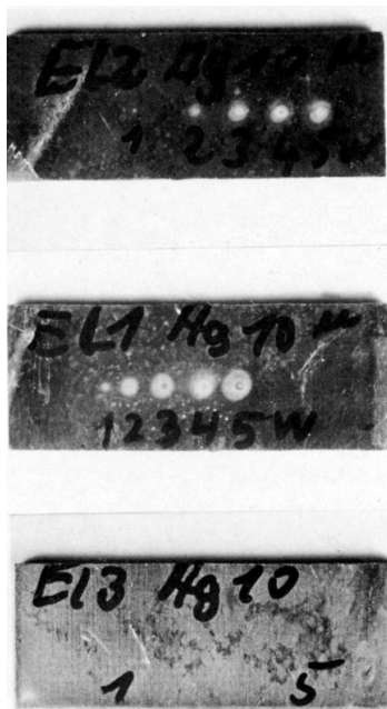
Figure 8 - Photos of laser-induced (at 1 to 5 W) gold deposits from (a) Bath EL2, (b) Bath EL1, and (c) Bath EL3 on 10- \mu m-thick silver. Magnification was 27 \times , 20 \times , and 31 \times for Deposits a-c, respectively.
