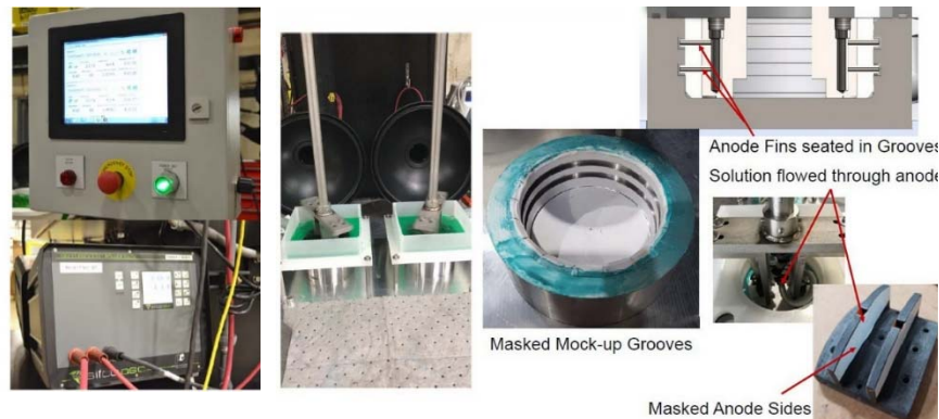
Figure 12- Automated ID plating, rectifier software and data logging.
