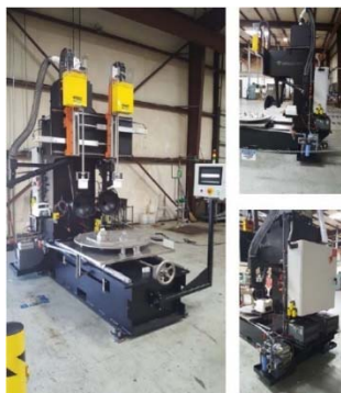
Figure 12- Automated ID plating, rectifier software and data logging.
