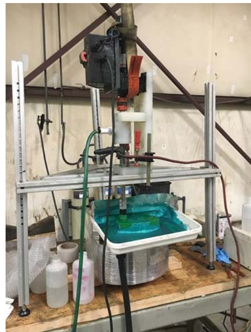
Figure 5 - Manual selective plating pilot apparatus: (L) rotating anode assembly; (R) complete pilot scale setup (vertical orientation).
