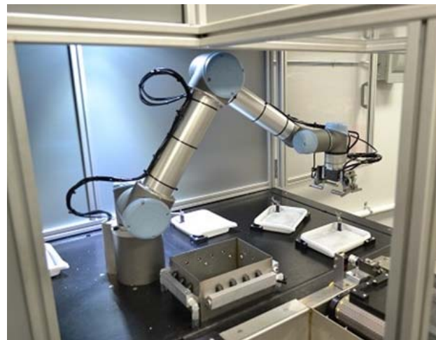
Figure 7 - Robotic selective plating system: (L) overall layout; (R) robotic handling arm and ancillary equipment.
