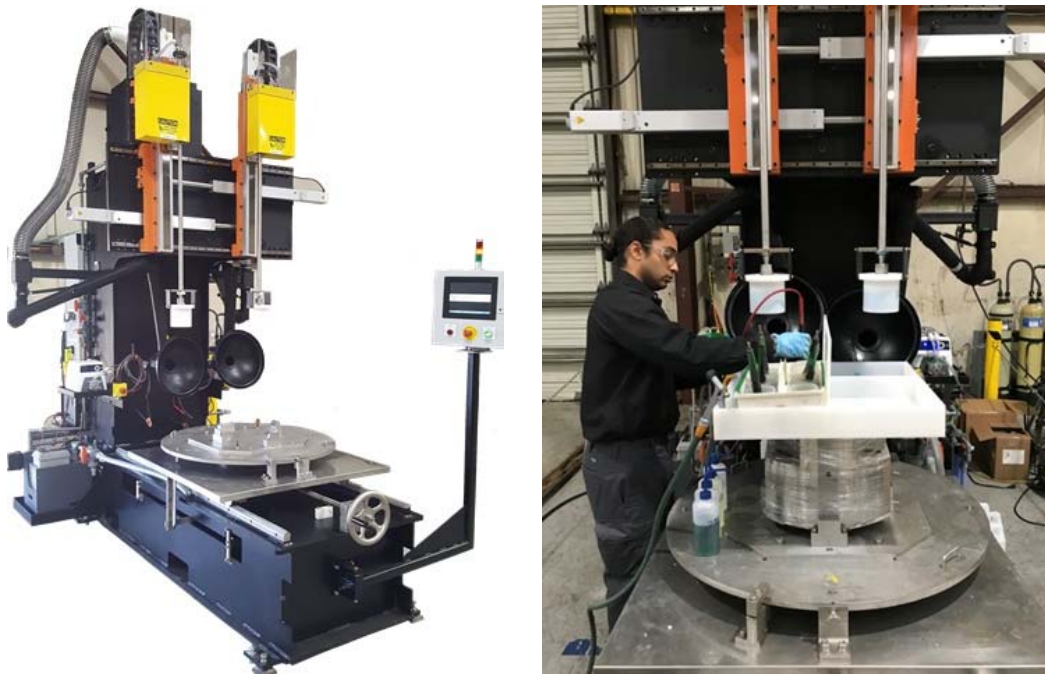
Figure 6 - Semi-automated machine for Ni plating of oil blowout preventer: (L) general view; (R) installation in operation.
