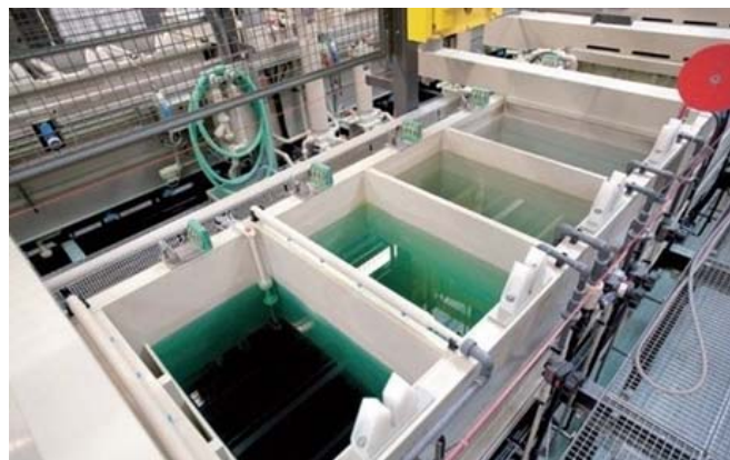
Figure 8 - Portion of a tank line for nickel plating Inconel turbine engine components.
