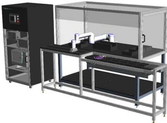
Figure 7 - Robotic selective plating system: (L) overall layout; (R) robotic handling arm and ancillary equipment.
