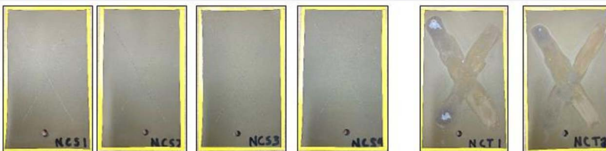
Figure 6 – Coated steel panels after 50-day U.S. Navy cyclic test. The first pair of panels in each row were coated with sacrificial basecoat alone (with no seal coat) and scribed, the second pair of panels were coated with sacrificial base coat and seal coat and then scribed, the third pair of panels were coated with sacrificial base coat, sealed, scribed and then touched up. Performance of Aseal 5KGT (lower row) was equal to or better than that of the legacy system (top row)
