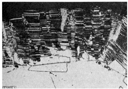
Figure 7 - Cross section of the BR-type (Cu deposited from acid CuSO<sub>4</sub> solution, magnification 250×).
