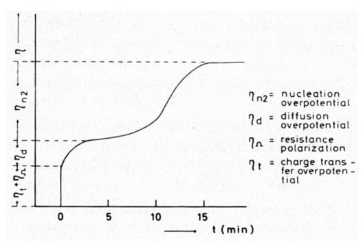
Figure 2 - Schematic curve of overpotential  $(\eta)$  versus time (t) with the single stages of overpotential during the deposition of copper in presence of an inhibitor (o-phenanthroline).
