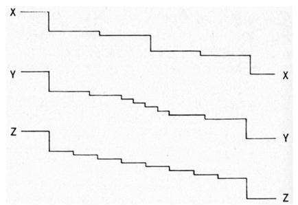
Figure 6 - Model for fading out of a macrostep from its end. (After Bockris and Razumney<sup>9</sup>).
