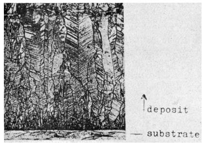
Figure 9 - Cross section of the TT-type (copper deposited from acid  $CuSO_4$  solution + 5 ×  $10^{-3}$  mol/L acridine, magnification  $600\times$ ).
