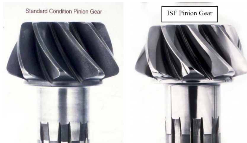
Figure 7 - Comparative results are shown for a pinion from a spiral bevel gearset for (Left) a traditional lapped finish versus (Right) the same pinion with an ISF finish.
