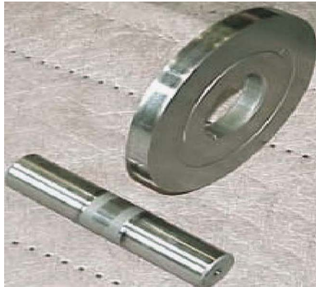
Figure 12 - A 1" diameter specimen pin at the lower left and a 5" loading roller at the upper right side of the photograph. 2,7
