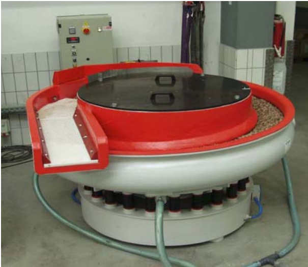
Figure 4 - A traditional vibrate bowl with parts/media separation deck; ideal for processing short stubby parts such as gears, tappets and bearings.
