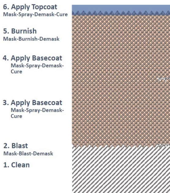
Figure 2 – Schematic of the chromate/phosphate system.
