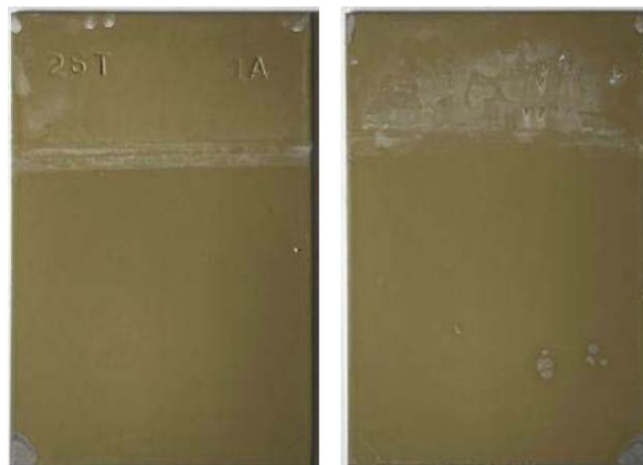
Figure 6 – Results of 1000 hr of hot water immersion test for Aseal™ REACH-compliant system.
