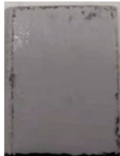
Figure 13 – Optical image of a 4-micron PEO surface on magnesium after deposition of 20-microns of Cirrus Polyshield™ topcoat.
