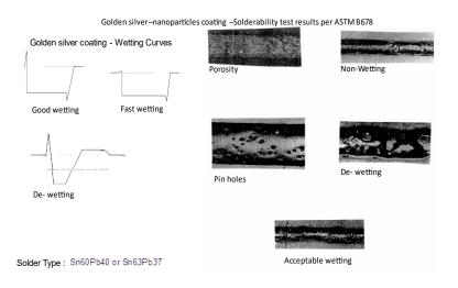
The Image #3 present the solderability test for golden silver material performed per Mil-STD-202 with the following acceptance criteria: Failure Criteria 5% maximum dewretted, nonwetted, or with pin holes. All passed.
