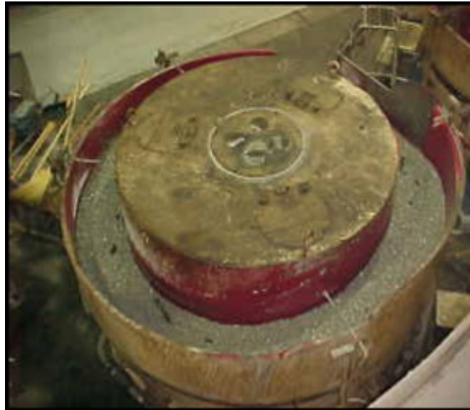
Figure 9 - Overhead view of a 40 ft 3 , long-radius style vibratory bowl.
