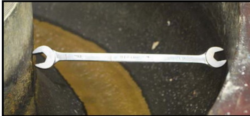
Figure 7 - A wrench jammed into a vibratory bowl channel.
