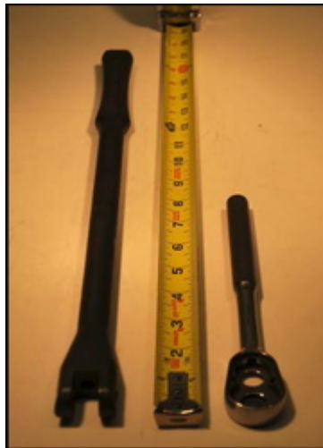
Figure 4 - Two parts being measured for length: 16.5 in. left-side part and 8 in. right-side part.
