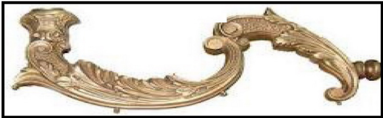
Figure 14 - A delicate, brass, chandelier trim piece that has been sand-casted and is to be vibratory processed to remove casting flash.
