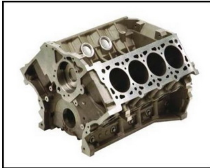
Figure 11 - A cast steel, automotive, V8 engine block weighing approximately 550 lb.
