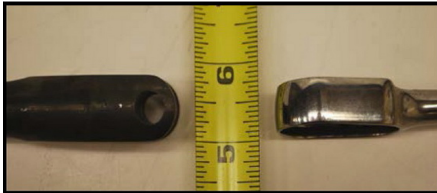
Figure 6 - Same two parts being measured for height: 0.75 in. left-side part and 0.625 in. right-side part.
