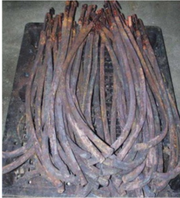
Figure 5 - Lead/tin anodes bent during plating.
