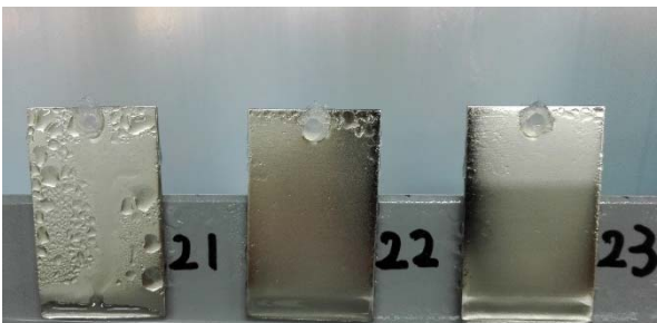
Figure 5 - 6-micron Hybrid Al 2 O 3 with semi-bright and bright nickel after 102 hr of salt spray testing.
