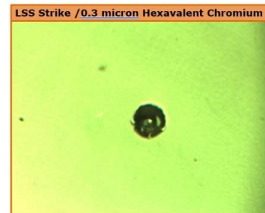
Figure 8 - Pit development after 88-hr CASS with a hexavalent chromium deposit over LSS nickel with very low porosity.
