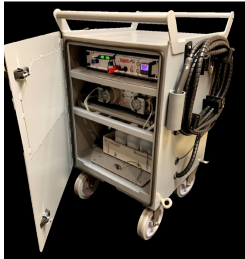
Commercial non-drip Ground Support Equipment for F-35 ZnNi repair
