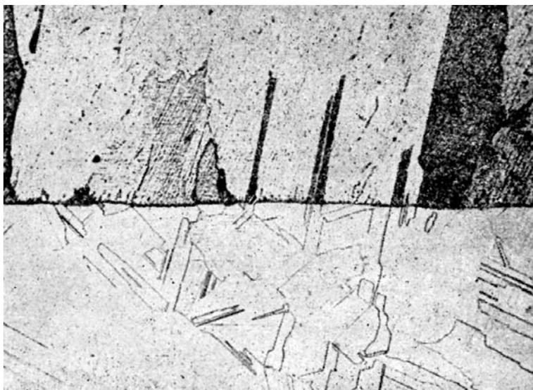
Figure 4 - Continuation of microstructure of annealed silver by electrodeposited copper: upper, copper deposit; lower, annealed silver.
