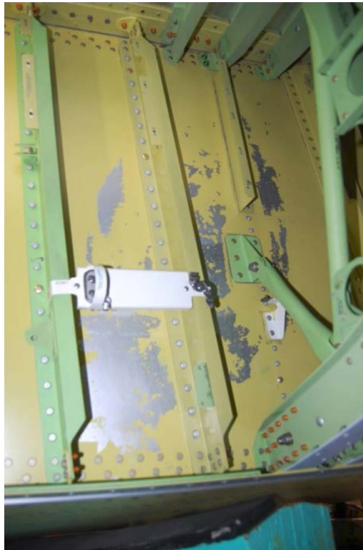
Figure 9 - Paint adhesion failure during assembly.
