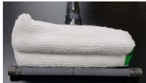
Figure 5 - Zn-Ni brush plating configuration.
