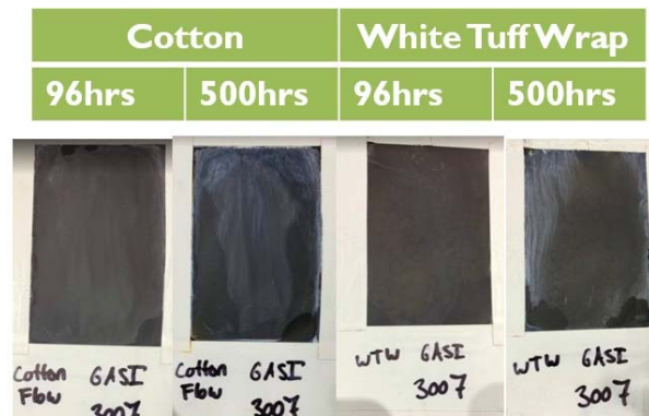
Figure 12- Best results from ASTM B117 testing.
