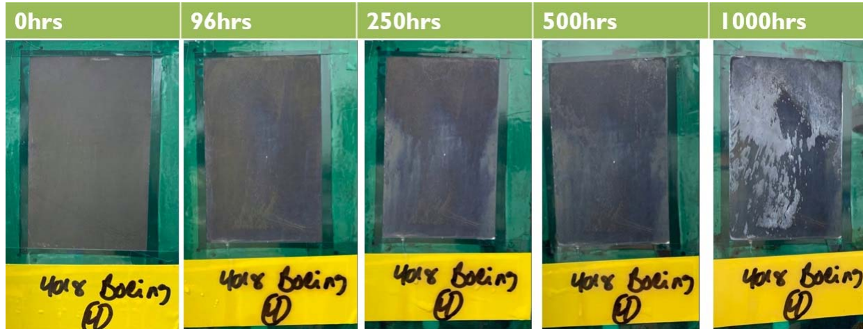
(a) Trivalent conversion coating applied by a 90-sec dip.
