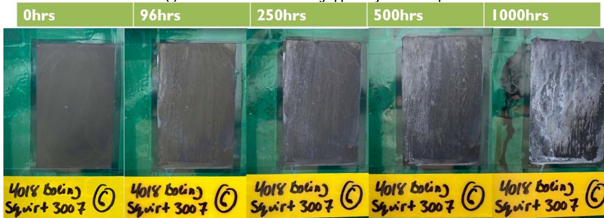
(b) Trivalent conversion coating applied by a 90-sec squirt/spray application.
